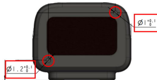
Figure. 4: Diagram of TF-NOVA installation hole
