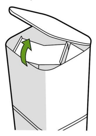
2. Pull up on the plastic card leading to the vacuum port and lift up to pull the *bag* out of the canister.
