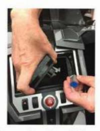
There are 4 sockets with 2 or more connectors attached to the back of the Head unit. Pay attention to where each these connectors attach, Unplug the connectors and remove the Head unit.
