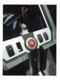
Once the head unit is removed, use a screw driver to pop out the factory rocker switch cap in your center console while pressing on the release clips on the side of the switch from behind.
