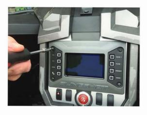
Start by removing the Head unit, there are 4 screws that will need to be take out.
