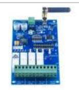
PCR43304R 4-Channel Receiver with Relay Outputs
