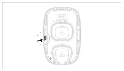
6. Reassemble Charge Amps Dawn by inserting the front cover bottom flange and rotate the cover in place. Secure in place by tightening the front cover lock screw using Torx 25.
