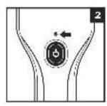
Plug the charging adapter into a wall cutlet. The charging indicator light will blink. Light will go out when fully charged.
