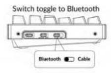
Press fn + 1 (for 4 seconds) and pair with device named Keychron K8
