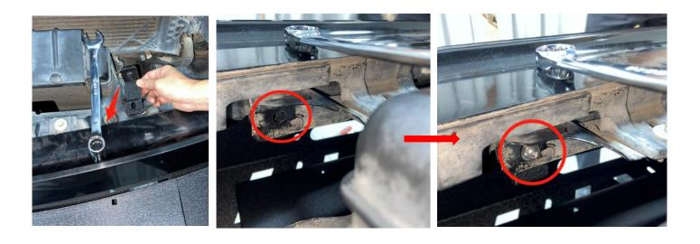
Step 8: Keep the bolts loose, raise the bumper, adjust the gap between it and the car, and then tighten up all of bolts after confirming that the desired effect is achieved.
