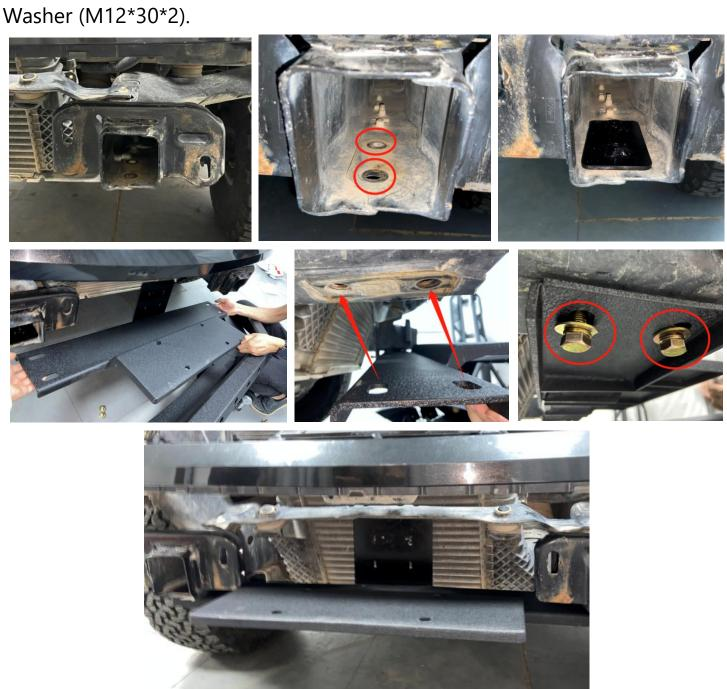
Step 6: Lift up the bumper and install it into your vehicle. Use the Hex Bolts (M12\*35), Split Lock Washer (D12), Flat Washer (M12\*30\*2), Hex Nuts (M12).
