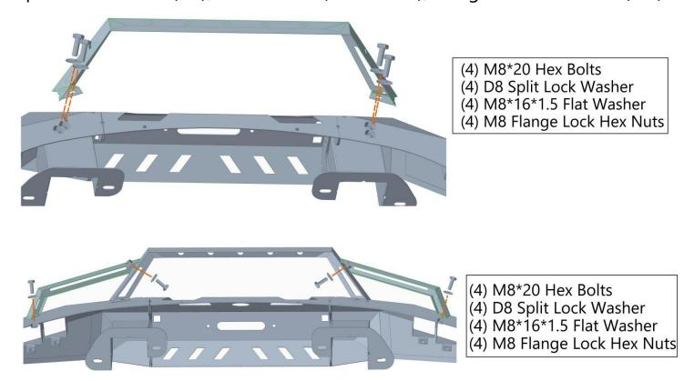
Step 4: To assemble the winch power control box bracket & the winch bracket. Use the Button Head Socket Cap Bolts Screws (M8\*20), Split Lock Washer (D8), Flat Washer (M8\*16\*1.5), Flange Hex Lock Nuts (M8). This step isn't 100% necessary. Depends if you have the winch power control box.
