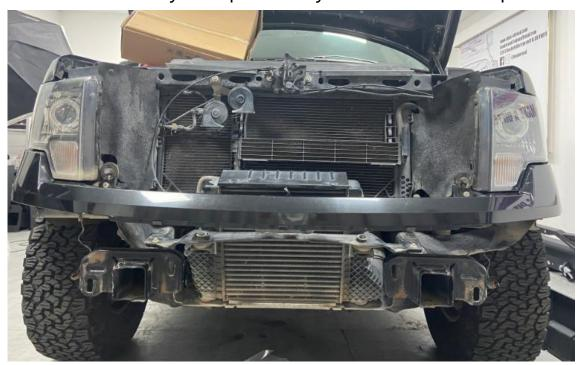
Step 2: To assemble the wings & the main body. Use the Hex Bolts (M12\*30), Split Lock Washer (D12), Flat Washer (M12\*30\*2), Hex Nuts (M12). Repeat the same installation methods in the other side.
