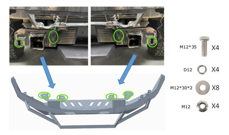
Step 7: To connect the bumper and the vehicle with the connect bracket. Use the Button Head Socket Cap Bolts Screws (M8\*20), Split Lock Washer (D8), Flat Washer (M8\*16\*1.5), Flange Hex Lock Nuts (M8). The upper bolts don't need install the flat washer & the split lock washer.
