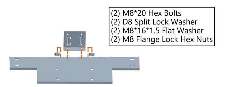
Step 5: Put the nut plate into the vehicle body. To install the winch bracket into the vehicle body. Use the Hex Bolts (M12\*30), Split Lock Washer (D12), Flat Washer (M12\*30\*2).
