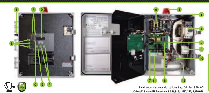
The IFS simplex control panel utilizes an innovative circuit board design to control one 208/240/480 VAC three phase pump in water and sewage applications. IFS panels feature an easy-to-use touch pad on inner door for programming and system monitoring. The panel configuration can be easily converted in the field to either a timed dose or demand dose. Available with the EZconnex® float system.
