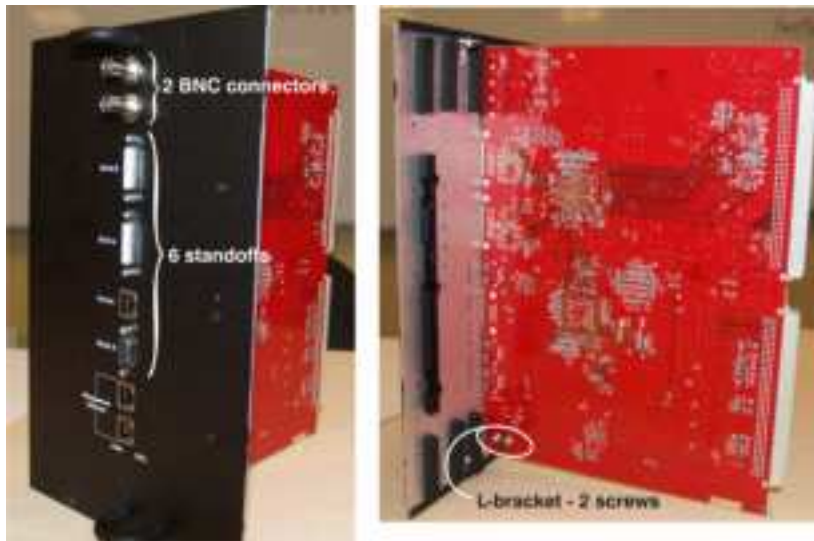
Figure 7 Separate ZX Faceplate from PCM
