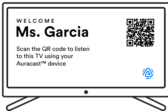
Figure 3.7: The use of QR codes to enable encrypted audio for hotel TVs
