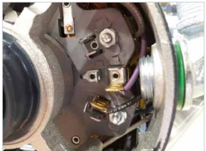
Line connection spades for L1, Neu (arrow 1 & 2)
