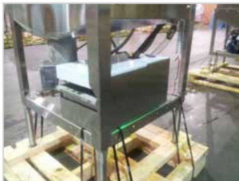
L-3DW-S scrap box in-frame mounting
