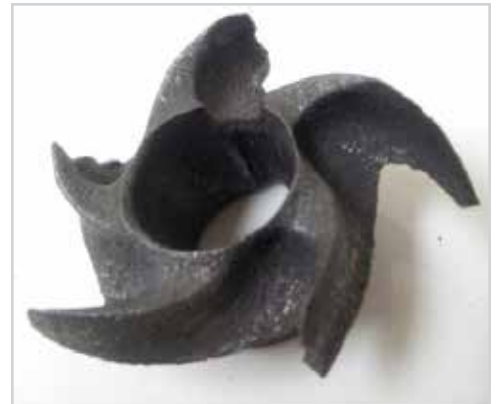
Impeller damaged from high acid solution
