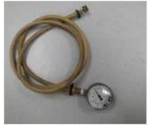
Spray arm pressure tester #088-1048
