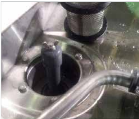
Showing sump, drain ball, pump filter
