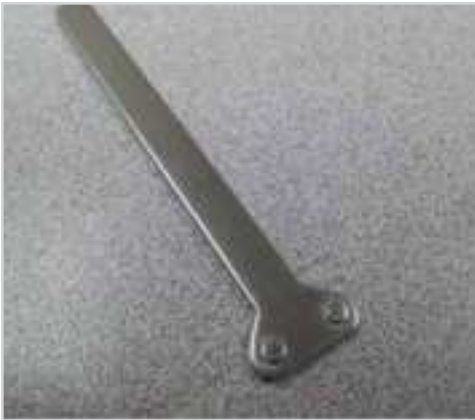
Cam timer adjustment tool
