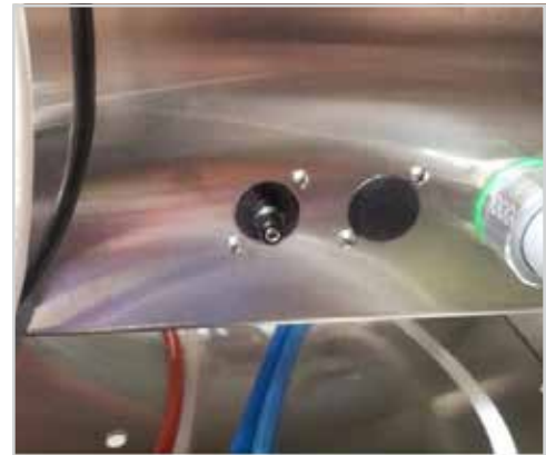
Chemical alarm barb adjusting screw*
