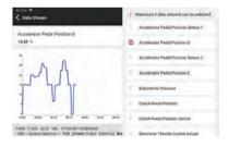
[Compare Sample] To select the sample DS file. All the values you customized and saved in process of DS sampling will be imported into the Standard Range column for your comparison.
