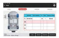
C. Learning: to write the sensor ID into the vehicle ECU for sensor identification.
