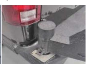
(Driver Side) Install the T-shaped pin to the carrier.
