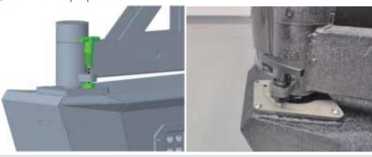
Install the adjustable latch to the carrier using the (6) M6x16mm button bolts, (6) M6x1x12mm flat washers, (2) M6 lock nuts. nuts.
