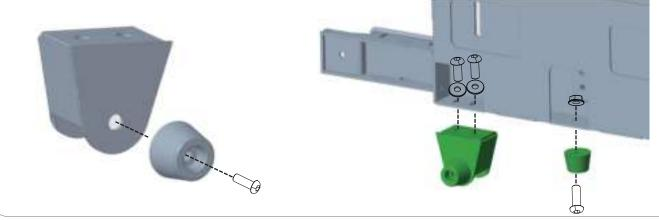
(Driver Side) Install the oil drum bracket to the carrier using the (4) M8x20mm button bolts, (4) M8x1.5x20mm flat washers, (4) M8 lock nuts.
