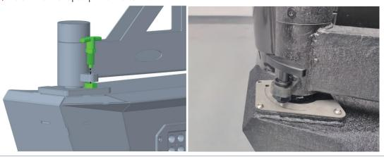
Install the adjustable latch to the carrier using the (6) M6x16mm button bolts, (6) M6x1x12mm flat washers, (2) M6 lock nuts. nuts.
