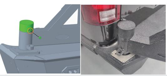
(Driver Side) Install the T-shaped pin to the carrier.
