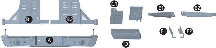
A: Bumper B1&B2: Carriers C1&C2: Spare Tire Mounting Brackets E1&E2: Reinforcement Brackets F1&F2: Nut Plates
