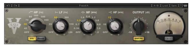
The Waves V-EQ3 Equalizer is three-band EQ with a highpass filter. Like the 1073 and 1066 hardware devices after which it was modeled, the V-EQ3 offers selected cutoff points and ±18 dB gain adjustment with a bell-shaped curve. The highpass filter can range from off to 360 Hz, with a slope of -18 dB per octave. Output gain can be adjusted up to ±18 dB.
