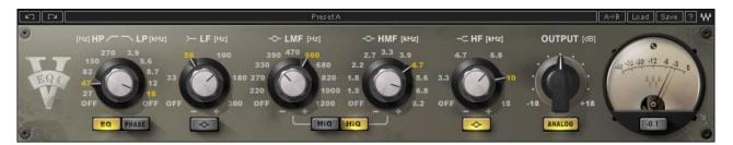
The Waves V-EQ4 EQ is a four-band equalizer with a lowpass/highpass filter. It was painstakingly modeled after the 1081 hardware EQ processor from the 1980s. Specific cutoff points provide great control while maintaining a warm, vintage sound. Like the V-EQ3, this EQ provides up to ±18 dB of gain adjustment, yet the V-EQ4 has switchable high Q settings, providing steeper EQ curves.
