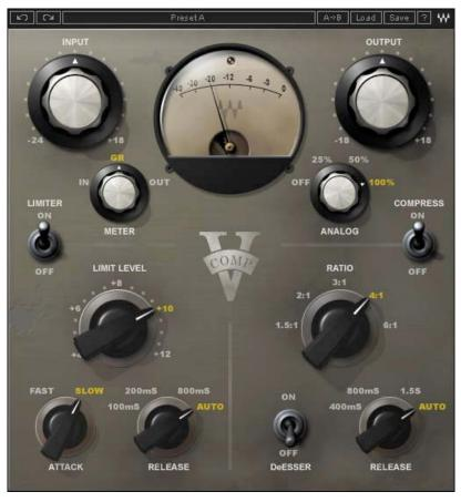
The Waves V-Comp Master Bus Compressor is a classic compressor/limiter with deesser. The V-Comp accurately models the renowned 2254 master bus limiter, providing very convincing vintage dynamic control.
