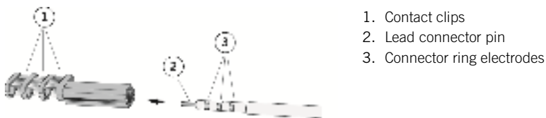
Figure 5. Inserting the lead into the connector sleeve
