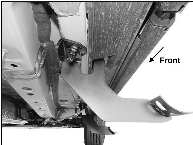
(Fig 17) Passenger/Right Center Bracket installed
