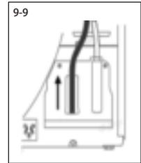
Uncoil the grey drain hose (included with your dryer) and connect it to the machine drain port (Fig. 9-10).
