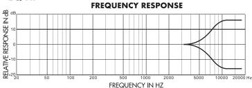
The high EQ control is a shelving EQ. What this means is that it boosts or cuts from 10kHz and everything above that. Turn it up to bring out the breath of a vocal or the high overtones of the cymbals. Turn it down to reduce finger squeaks on a guitar or bass.
