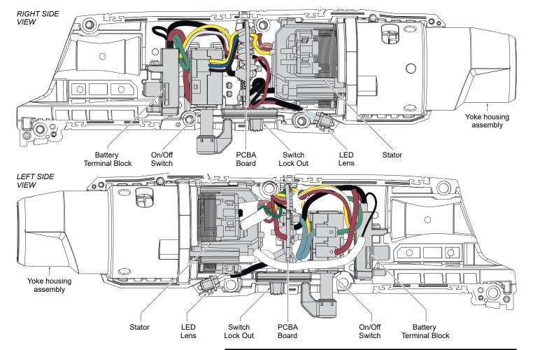
SEE NEXT PAGE FOR SERVICE INSTRUCTIONS TO AID WITH THE REMOVAL AND INSTALLATION OF ELECTRONICS ASSEMBLY (104).
