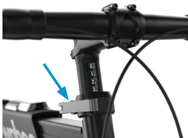
Stack Height Adjustment
