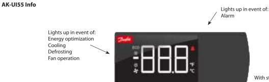
With start-up /connection to a controller, the display will "light up in circles" as it collects data from the controller.
