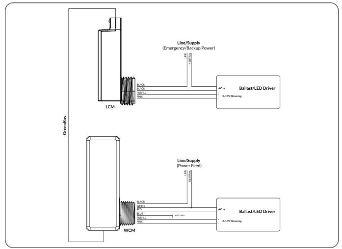
Note: Please refer to LCM wiring and installation manual (included with applicable product) for connection information. As the LCM is not supported by the Encelium Edge System, this is only available with the Encelium X Networked System.
