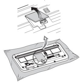
3 Insert the four new batteries, being careful to follow the polarity markings on the inside of the compartment.
