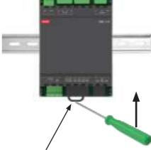
Pull stirrup using screwdriver and remove EKE from rail
