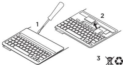
1. Pry off top cover of keyboard with screwdriver.
