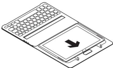
2. At the bottom of the tablet holder, use the two rubber bands to fix the tablet in place:
