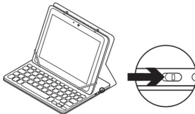
The status light blinks blue to indicate that the keyboard is discoverable, ready for pairing with your tablet. The first time you turn on the keyboard it remains discoverable for 15 minutes. If the status light turns red, charge the battery. For more information, see "Charging the keyboard battery."
