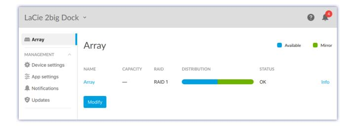
Click Array to view the capacity and status of the disks in the array.
