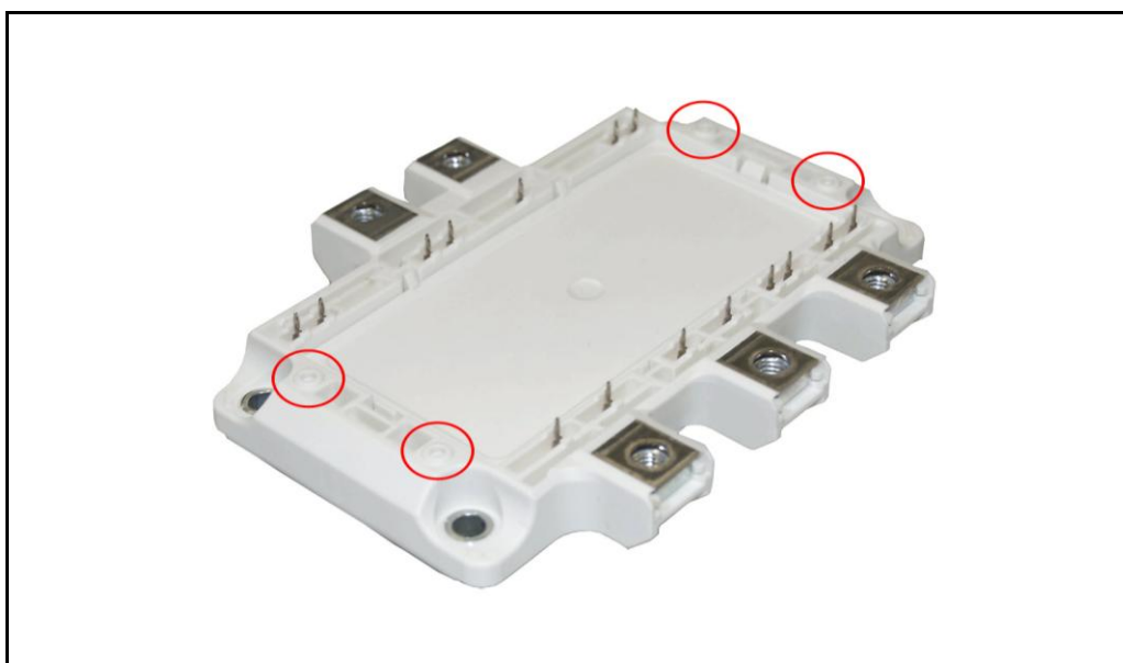
Figure 4 PCB mounting stand-offs of EconoPACK™ 4 modules (marked red)
