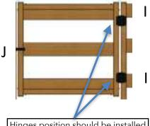
Hinges position should be installed 2.5" inches from the top and bottom of the U-Post.
