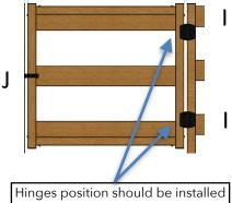
Hinges position should be installe 2.5" inches from the top and bottom of the U-Post.
