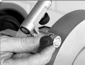
Remove the knife jig from the machine and replace it with the RBS-140 Round Blade Sharpening Attachment (hereafter referred to as the "Accessory").
