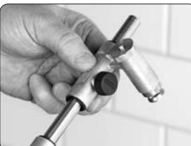
To set the size, loosen the guide's stop screw and slide it to the desired size. Tighten the stop screw again to lock.
