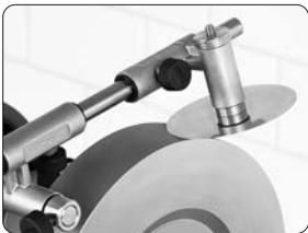
Fold down the Accessory so that the blade's bevel is against the diamond grinding wheel and start the machine. Blade sharpening now begins.
