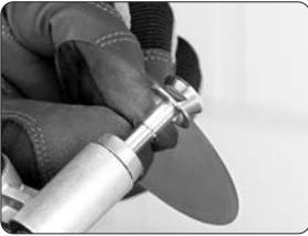
Thread the tensioner through the blade hole with the bevel against the thick end. Refit the tensioner and the blade in the guide.
