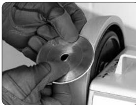
**⚠ Use protective gloves to help prevent cuts! Ensure that the honing wheel rotates **from** the edge, otherwise the blade will cut into the honing wheel.**
