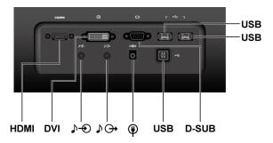
3. Connect one end of the analog signal cable to the monitor D-Sub connector and the other end to the computer.
