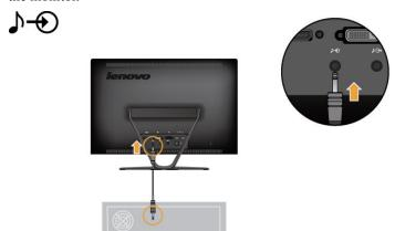
8. Connect the headphone to the headphone output terminal of the monitor.
