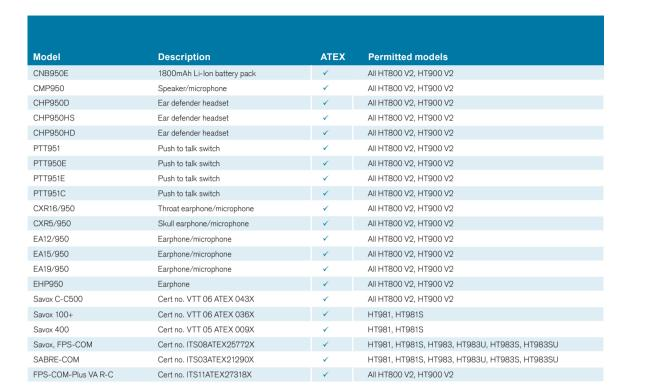
The Entel ATEX transceivers should only be used with the specific, permitted accessories, as detailed above.
