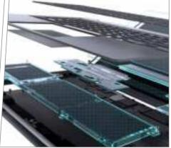
ASUS BR1100 has a modular design that allows key components — such as the keyboard, battery, thermal module and I/O ports — to be replaced in minutes using simple tools.
