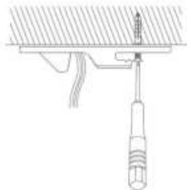
5) Align the bracket at the bottom of the device with the bracket buckle, and push the product in the opposite direction of the bracket hooks until it is buckled tight (make sure the power cable or Ethernet cable is properly connected before it is tightened).
