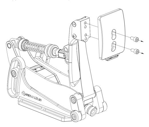
Add the foot support between the pedal arm and pedal face. Use the new bolts supplied (A2) to secure all parts.
