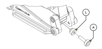
Adjusting spring force isn't only possible by using the adjustment knobs. Using the lower of the three adjustment holes on the pedal arm gives you a slightly softer (S) pedal pressure for example. The higher of the three a slightly firmer (F).
