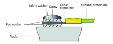
FIG. 7 Grounding protection diagram
