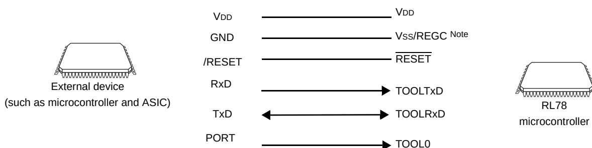
Figure 30 - 4 Communication with External Device
