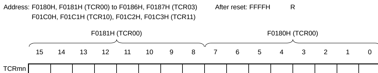
Figure 6 - 9 Format of Timer counter register mn (TCRmn)
