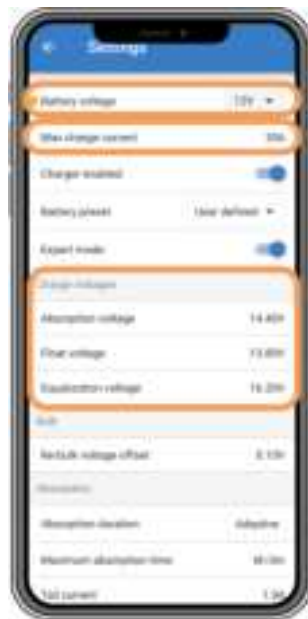
VictronConnect app, showing battery (system) voltage, charge current and charge voltages settings.
