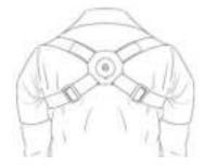
5. When the device detects the user leaning forward, both vibrators vibrate simultaneously; when leaning to the left, the left vibrator vibrates; and when leaning to the right, the right vibrator vibrates.
