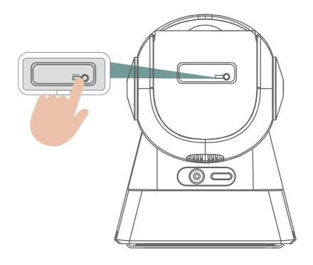
1. Press and hold "Reset" for more than five seconds to Reset the device;
