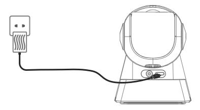
Please charge the Battery Camera with the included power adapter for at least 5 hours.
