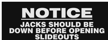
Fig. 4.1 Leveling jack label
