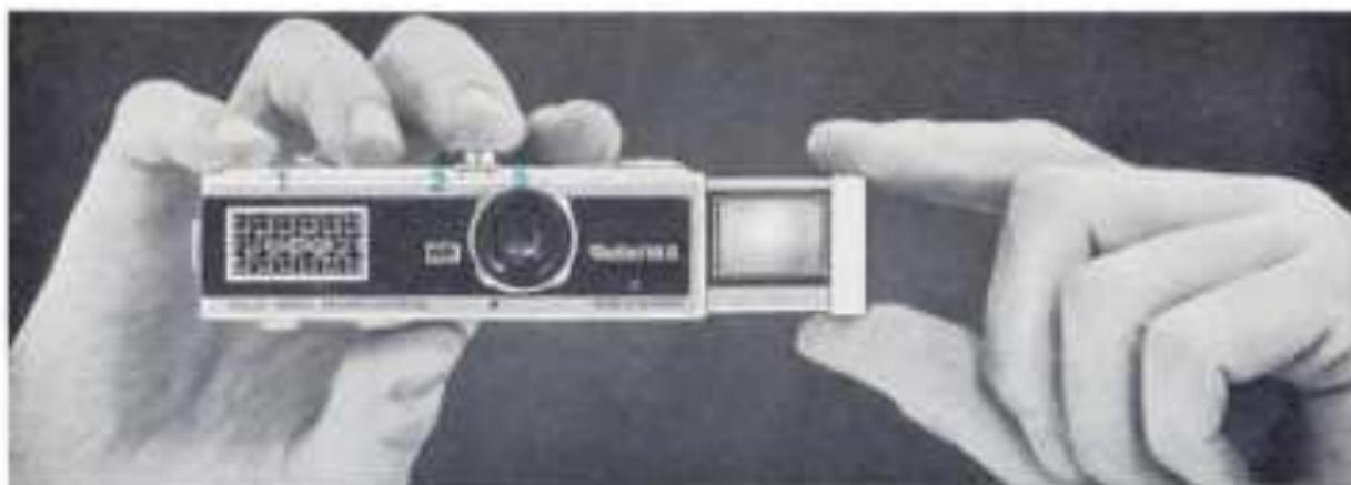
The exposure control system is coupled with the special shutter of the Rollei 16 S. It controls the automatic selection of shutter speed and aperture according to the measured exposure value.
