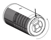
Twist the bottom panel counterclockwise to remove the panel.
