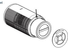
3) Remove the old filter and dispose of it properly. The filter is not recyclable.
