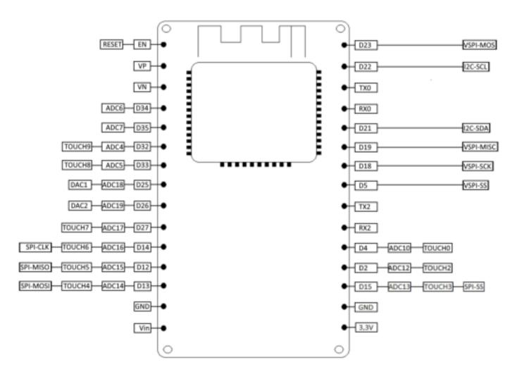
The input voltage via USB-C is 5 V ±5%. The input voltage via Vin-Pin is 6 - 12 V.
