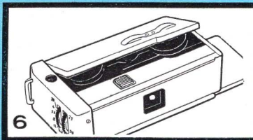
6. If door does not close, it is because magazine has not gone all the way in.
