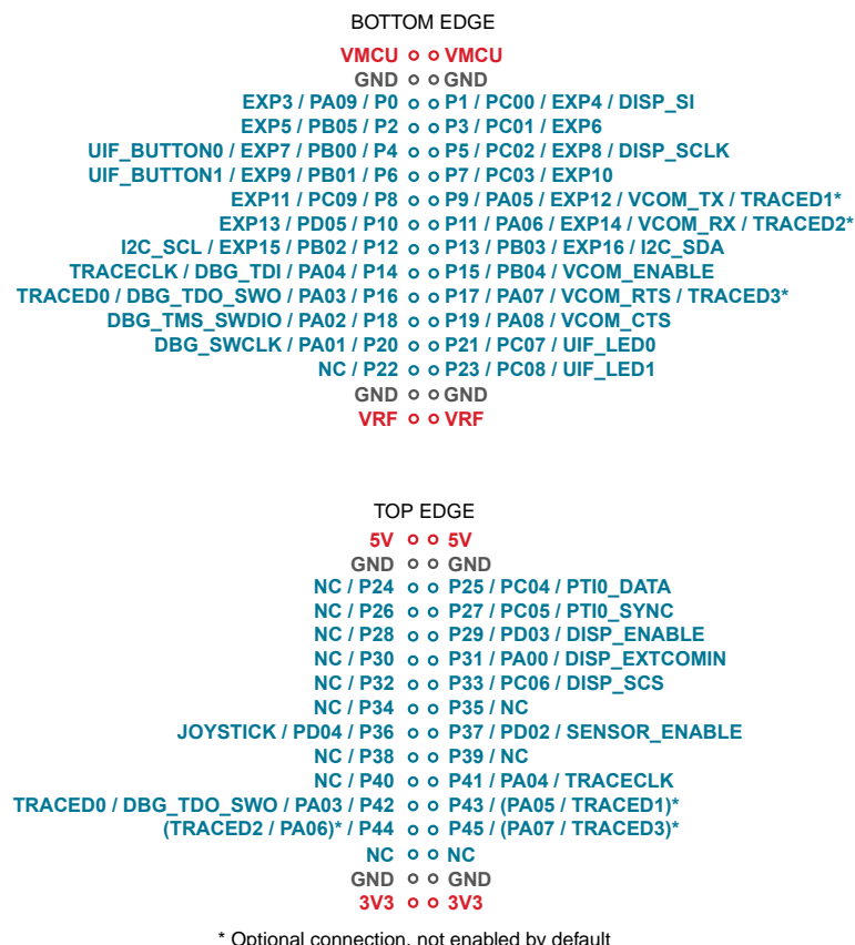
Figure 3.4. Wireless STK Mainboard (BRD4001A) Breakout Pad Pin Mapping
