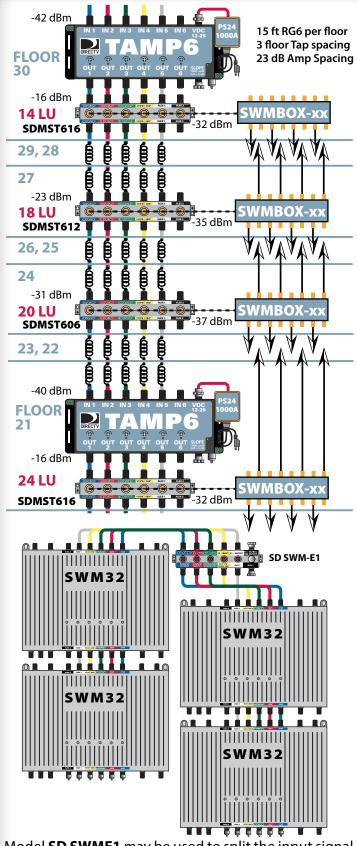
Model **SD SWME1** may be used to split the input signal to (2) sets of **SWM32** switches. The minimum input to the **SD SWME1** is -40 dBm so that each **SWM32** has a minimum of -45 dBm.
