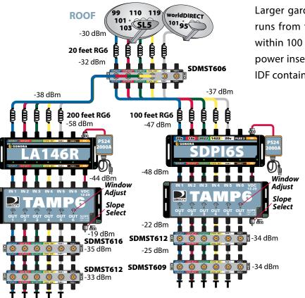
Larger garden style MDU buildings may have longer runs from the dish to the IDF closets. Place the dish within 100 feet of the IDF containing model **SDPI6S-T** power inserter. The thru port of the coupler feeds the IDF containing the **SDPI6S-T** power inserter.
