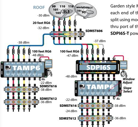
Garden style MDU buildings often have IDF closets at each end of the building. The signal from the dish is split using model **SD MST606** directional coupler. The thru port of the coupler feeds the IDF containing the **SDPI6S-T** power inserter.
