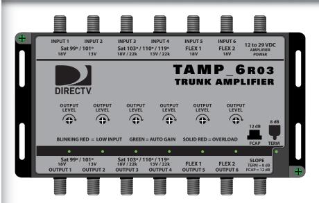
Model **TAMP6R03** provides either 8 dB or 12 dB of cable slope pre-emphasis. A weather sealed F cap is shipped on the units lower right F connector.
